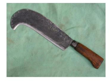
This is used (with a mallet/beetle) for splitting green wood
